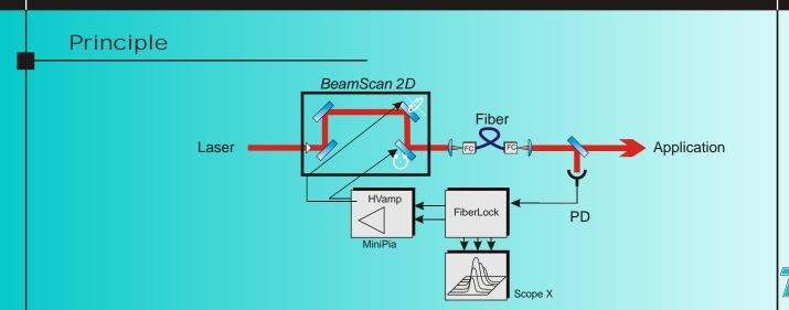
Usually, the coupling into single-mode fibers is a time-consuming task since mechanical positioning with sub-micrometer precision has to be performed. Expensive moving or tilting units with very good long-term stability have to be used.
