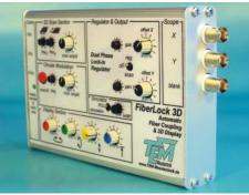
*FiberLock 3D:* Scan and Regulation Electronics
