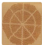
Textile, 10 pulse per pore mean power 1 W, 800 Hz
