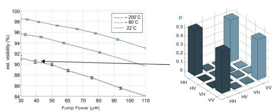
Expected TPI visibility as a function of computer-controlled pump power at various fiber temperatures. Two-photon generation rate improves quadratically with pump power, but due to multiphoton effects the quality of entanglement degrades, lowering the TPI visibility.
