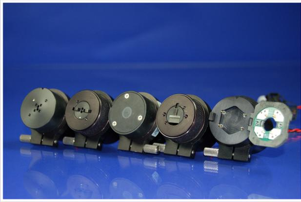
The OL 700-80 series of LED holders, adapters and alignment jigs, interface a large range of leaded and surface mount LEDs with Gooch & Housego's state of the art photometers and spectroradiometers.
