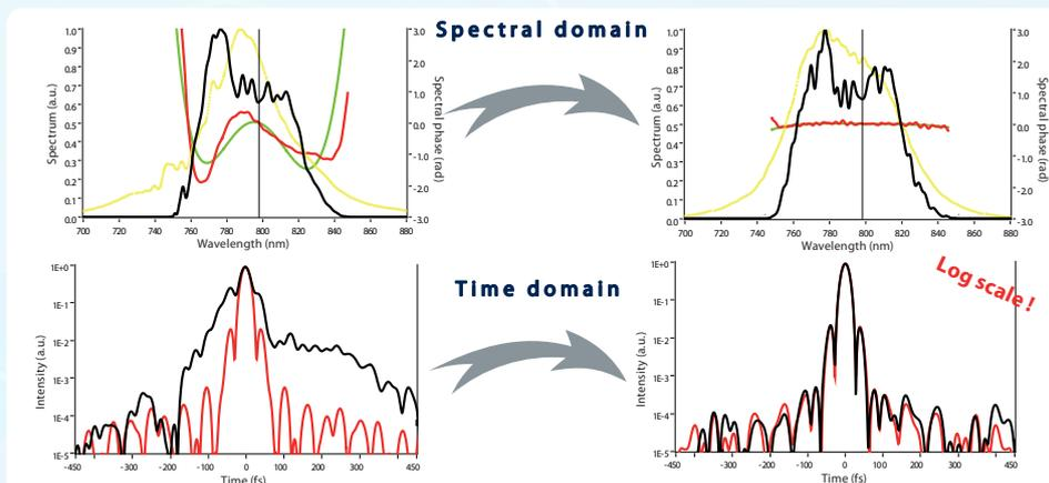
Wizzler measurements of a Ti:Sa amplifier (1kHz, 1mJ, 25fs FWHM) before and after the Dazzler / Wizzler feedback loop.
