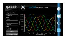
Polarization entangled states show correlations for all different combinations of the polarizer settings. You can fix one polarizer at 0° (horizontal, in the screenshot red), 45° (yellow), 90° (vertical, blue), 135° (green). The other polarizer is rotated. This shows the "non-classical" correlations of entangled photons.
