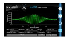
In a Michelson interferometer, the light is split up at a beam splitters into two arms and combined again and it will show interference. You can show that this is also possible with single photons. Perform this experiment with the quED and its add-on for the Michelson interferometer.
