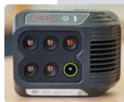
Configuration: 5 lens 8mm + 1 lens 4,2mm
