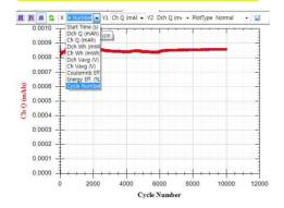
• X and Y-axis: Start time, Dch/Ch Q, Dch/Ch Wh, Dch/Ch Vavg, Coulomnb/Energy efficiency, Cycle Number
