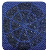
Textile, 25 pulse per pore mean power 1 W, 800 Hz
