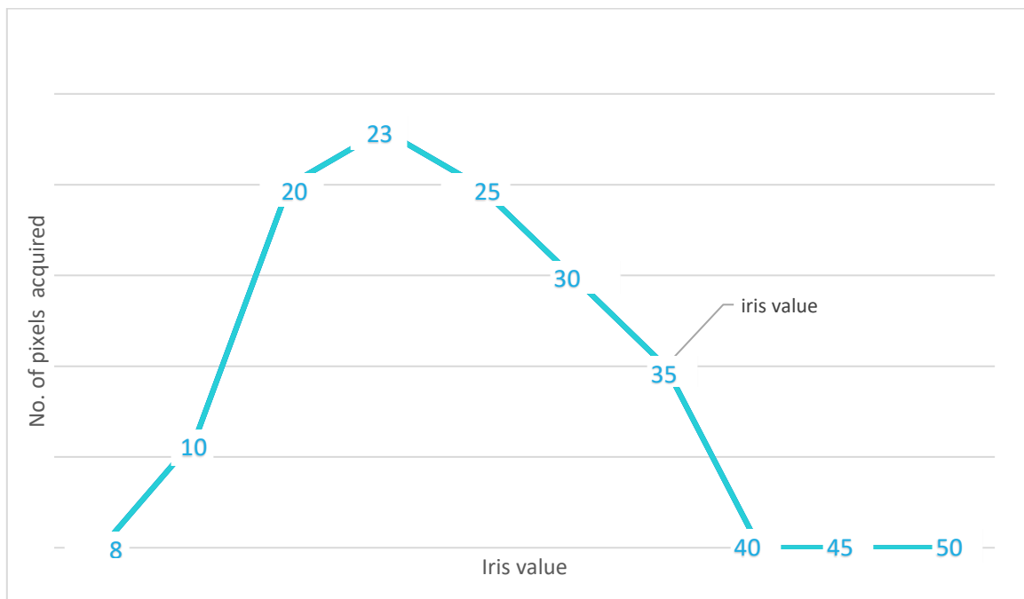
Fig. 1.8 Number of pixels acquired and iris value for a white sample object
