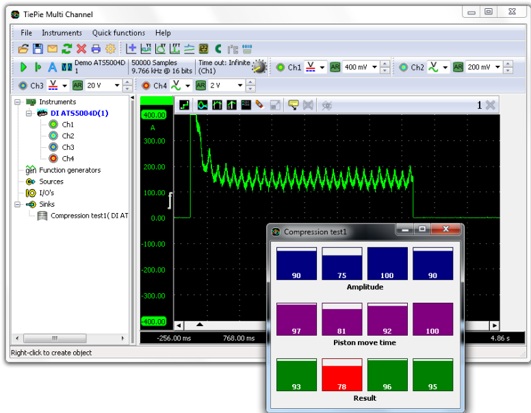
Figure 9.5: Compression test on engine with leaking cylinder
