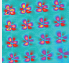
FeCr Ferromagnetic Nanostructures, 6.5 \times 6.5\mu\text{m}
