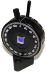
Manual polarizer for each arm of the entangled photon pair source.
