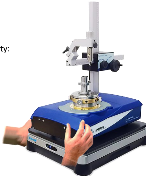
Figure 3-6 Center and level equipment on top plate
