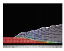
In the above experiment the motion of the different quartz sand layers was measured by a strainmaster system (incorporating pco.pixelfly cameras) and the strain field was computed, courtesy of LaVision, Göttingen, Germany
