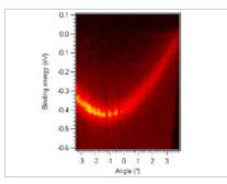
Cu (111) state dispersion image by a pco. pixelfly, courtesy of Specs GmbH - Surface Analysis and Computer Technology, Berlin, Germany
