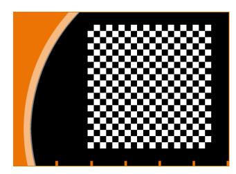
A checkerboard with a total size of  $9.0 \times 9.0 \, \text{mm}^2$  out of  $50 \times 50 \, \mu \text{m}^2$  squares. It is particularly suitable for testing of image skew and curvature. The edges are extremely straight and sharp and therefore allow determination of local image quality as well.
