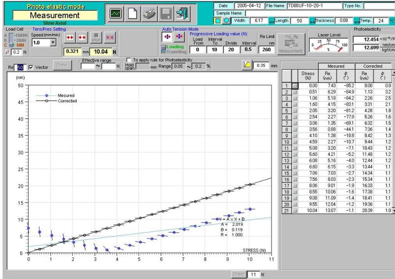
应变变量VS延迟TAC (三乙酰纤维素) 薄膜
