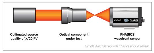
Applies to lens, objective, zoom, strongly aberrated subassembly.
