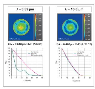
Chromatic behaviour measured with one unique sensor on a ZnSe lens of 25.4 mm diameter. The focal spot shifts 560 µm due to refractive index dispersion.
