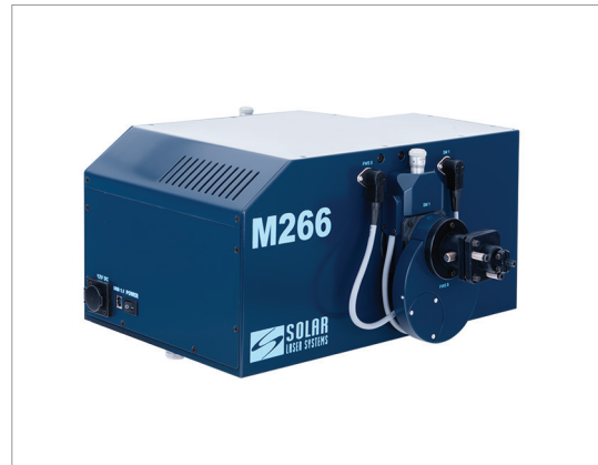
Monochromator M266i is fully automated, can contain up to 4 gratings; it's focal length is twice of M150i. It allows to open the slit two times wider for specified bandwidth of spectral range, and thus optical power is 4 times larger.
