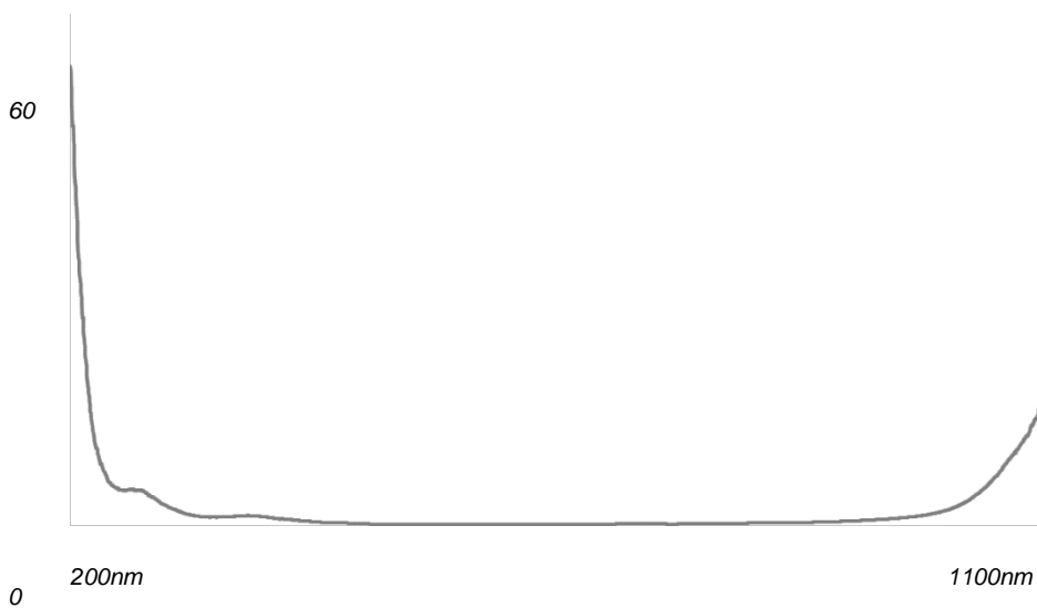
Typical cosine corrector calibration correction factors.
