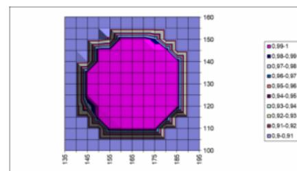
The ISS-17-VA offers an excellent uniformity of the Luminance distribution of typical  $\pm 0,5\%$  to the center point and  $\pm 0,3\%$  to the average value. The diffuser UMPF-LSOK30-DTB was used during the measurement of sphere homogeneity.
