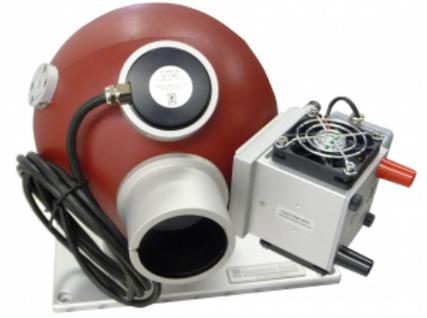
ISS-17-VA with reference detector
