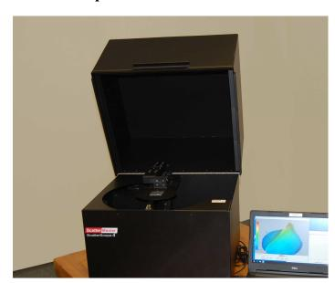
TSW is proud to announce the SS4 scatterometer. This patented instrument is a new concept in high-speed scatter metrology. It operates in both reflection and transmission and provides BRDF measurements in seconds instead.
