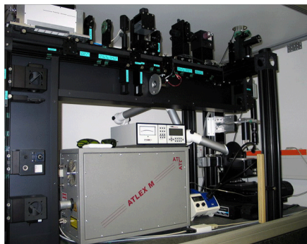
Micromachining System based on ATLEX-S-193 nm Short Pulse Excimer Laser (Courtesy of FZK, Karlsruhe)
