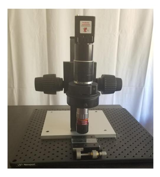
We can mount the microscope optical train onto a standard optical breadboard which will have an array of ¼-20" or M5 threaded holes (left image). With this mounting the user will have great flexibility is selecting and mounting standard translation stages to move the sample in X-Y-Z direction with micron position. Motorized stages and light sources can be easily mounted to the microscope breadboard and replaced quickly with components needed for the particular application.
