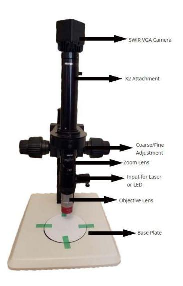
Your target sample may emit SWIR light naturally or when it is illuminated by an external light such as an LED or laser. You must know ahead of purchasing a configuration what spectral range you need to image. The most common configurations will support imaging between 900-1700 nm. If spectral imaging requirement is broader than 900-1700 nm, the cost of the microscope will increase quite a bit.
