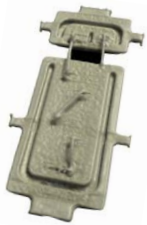
1.5 mm LED reconstructed using KA Imaging's inCiTe™ micro-CT.
