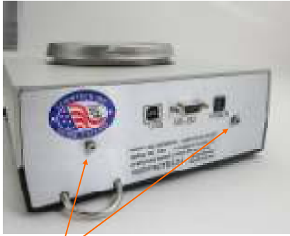
Disconnect power. Remove two screws. Pull panel out to gain access to calibration jumper. (Figure 1)
