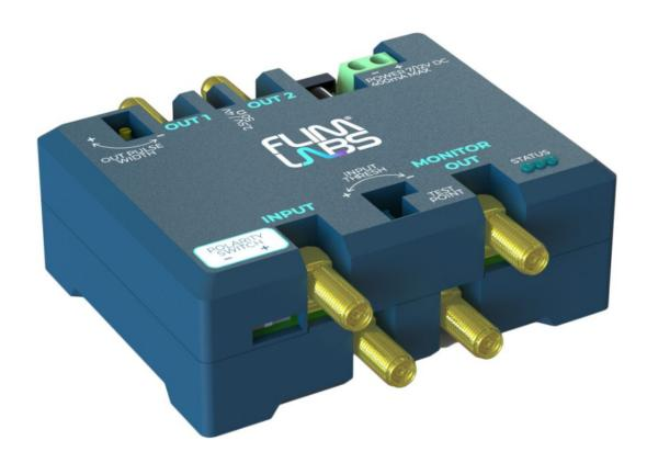
A constant fraction discriminator (CFD) is an electronic device that generates digital exact time stamps for input signals having changing amplitudes but a constant rise time.
