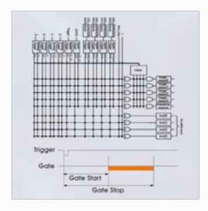
A multitude of useful details help you to create a highly integrated setup with a minimum of external components. Using the integrated TiGer timing pattern generator can provide digital pulse patterns to control your experiment or internal triggers. Use gate and veto functions with our gating logic. This also works across channels or from the additional digital input with a flexible trigger matrix.
