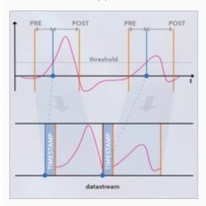
Detect pulses above a certain threshold and only acquire the relevant data to massively reduce the amount of data that needs to be copied and analysed.
