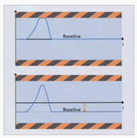
When acquiring unipolar pulses, shift the baseline to the edge of the ADC range to double your dynamic range compared with conventional ADC boards.
