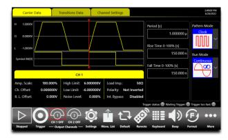
The software architecture provides the possibility to easily generate the patterns in different generation modality and also gives the opportunity to modulate the patterns with internal or external signals with the purpose to generate also different effects of noise (jitter, ripple, ...).
