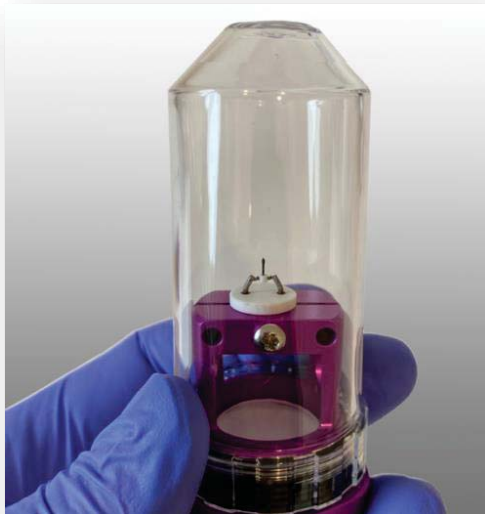
Cathode transporter with anodized aluminum base and sealable clear cover to protect the cathode during storage and transport. This example shows cathode ES-423E, a LaB 6 single crystal mounted on the end of a single piece of carbon heater rod, with a carbon ferrule to secure the LaB 6 .
