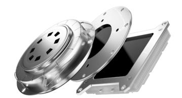
The singularity of Z-stack MCP is that it has spaces between microchannel plates (having separate supplies) and it makes it possible to obtain the gain of more than  $1\times10^7$  (shevron) and  $1\times10^9$  (Z-stack) in contrast to other similar assemblies which do not have spaces between the plates and have the gain of  $1\times10^6$  and  $1\times10^8$  respectively.
