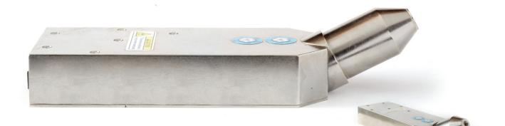
**Model M54:** 50 kV, 4W X-ray Monoblock - The M54 x-ray monoblock is a fully integrated miniature 50 kV, 4W x-ray generator designed specifically to be used as component of a handheld, portable, or benchtop x-ray instrument. The source includes a miniature sealed x-ray tube with a transmission-type end window, a high voltage power supply, and control electronics contained in a compact grounded enclosure.
