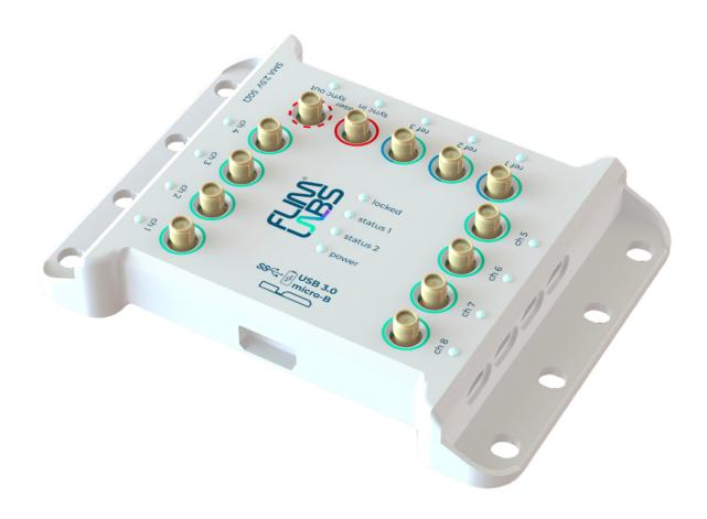
Our compact, USB-powered data acquisition card is designed for fluorescence lifetime imaging and spectroscopy measurements. It is portable and its features embody FLIM LABS expertise and mission.
