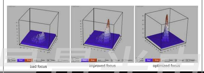
**Lock**: Once an intensity peak is found, the *FiberLock* can lock the piezo scanner to the point of maximum coupling efficiency. This is done with small circular modulations of the scanner angle and 2D lock-in regulator. While in lock, other degrees of freedom (e.g. the focus) can be optimized "live" in a fast and convenient way.
