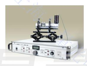
The LASS-II (Laser Amplitude Stabilization System) is an electro-optic feedback loop designed to reduce amplitude variations commonly associated with most gas lasers. This system is capable of significantly enhancing the signal/noise ratio of the laser over a much broader bandwidth than typical optically coupled current modulation of the plasma tube. Both an internal and external reference input is provided, allowing analog programming of the laser throughput. This is particularly convenient for
