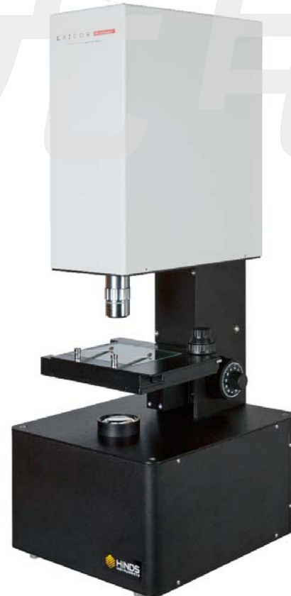
Figure 2. The Exicor Birefringence MicroImager. Footprint is 12 inches X 10 inches (30.5 cm X 25.4 cm) Height is 27 inches (68.5 cm)
