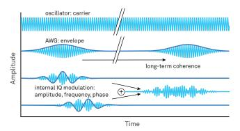
The HDAWG is equipped with digital oscillators to generate the sinusoidal carrier of a signal independently of the programmed AWG envelope signal. This means that long signals can be generated with very fast waveform upload and precise phase coherence across many pulses. Carrier frequencies and phases that would otherwise be written to a static waveform can be freely adjusted and swept.
