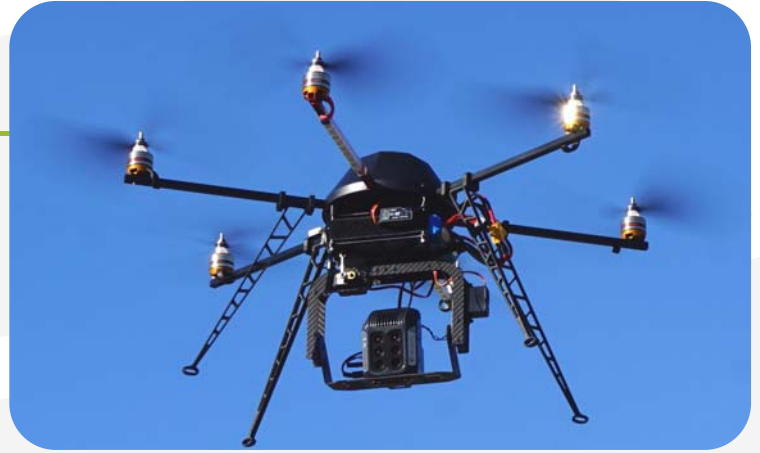
AIRPHEN embedded on UAV
