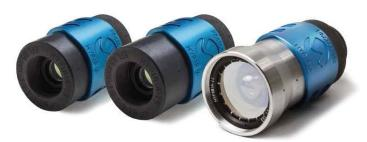
The HypIRia are telecentric objective lenses optimized for 1 to  $2.9~\mu m$ . They deliver a high throughput for high-quality imaging. Three different focal lengths are available: 25.3~mm (HypIRia 25), 15~mm (HypIRia 15) and 11~mm (HypIRia 11). Those lenses possess a broadband anti-reflective coating to reduce stray light and maximize the throughput.
