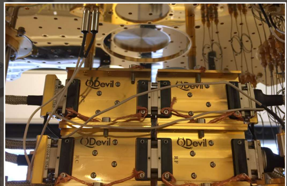
QFilters can be mated and stacked. For in-series mating filters are usually ordered in pairs: one filter with two RF banks and one filter with two RC banks.
