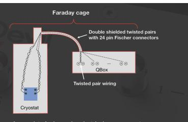
Appropriate for low-noise electrical measurements, the QBox and the Fischer cable extend the Faraday cage of the cryostat to the BNC panel.
