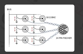
All BNC connectors are connected pair wise, using twisted leads, to the 24 pin Fischer receptacle. Each channel can be grounded or connected to common bus (BUS).
