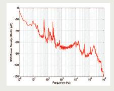
The phase noise power spectral density of the laser.
