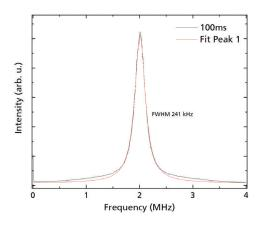
100 ms beatnote with Ti:Sapphire laser measured to have 160 kHz linewidth. Lorentzian fit has FWHM 241 kHz. REMOTE-Rb linewidth from this plot is 81 kHz @ 100 ms (locking to Fabry-Pérot interferometer, >200 finesse 1.5GHz FSR).
