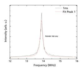
1 ms beatnote with Ti:Sapphire laser measured to have 110 kHz linewidth. Lorentzian fit has FWHM 190 kHz. REMOTE-Rb linewidth from this plot is 80 kHz @ 1 ms (locking to Fabry-Pérot interferometer, >200 finesse 1.5GHz FSR).
