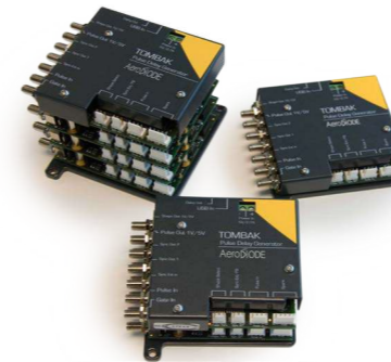
Possibility to stack multiple synchronized modules.
