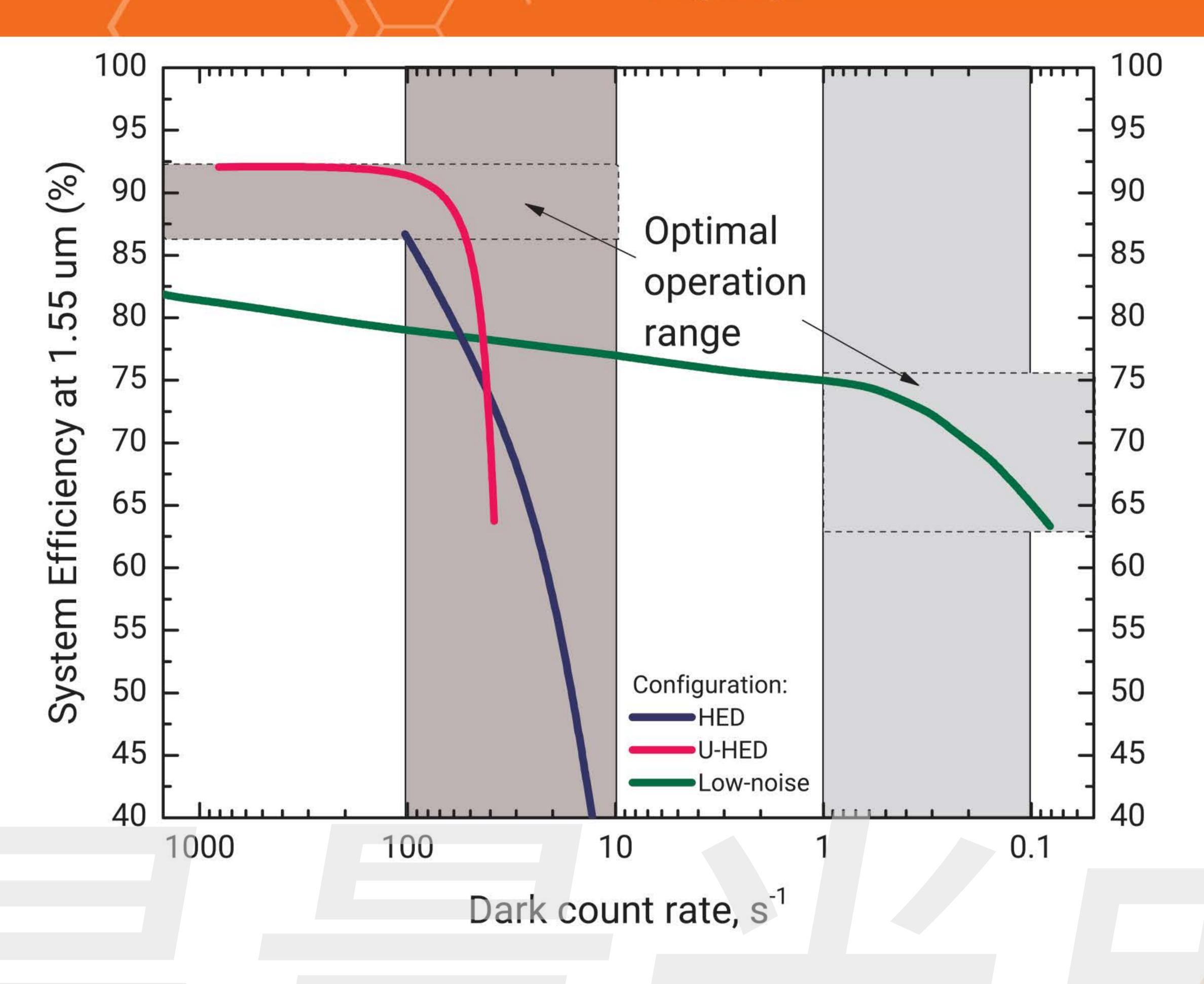
In SSPDs, system efficiency, dark count rate and photon energy establish the performance of the device. There is always a trade-off between reaching the highest efficiency and keeping the noise level low. For lower photon energies this relation is more prominent. To adjust the detector efficiency it is possible to vary its bias current as shown below.
