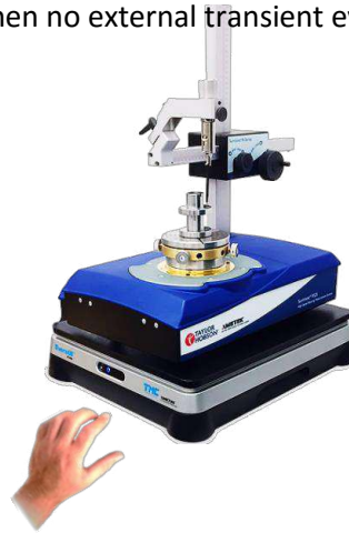
Figure 3-7 System automatically levels top plate
