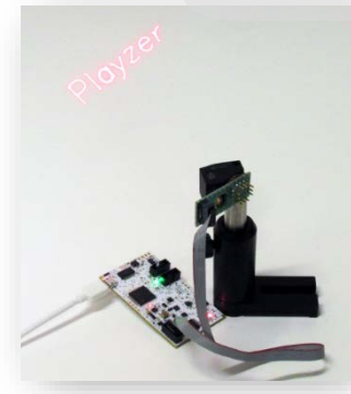
Example application of a Scan Module in Vector Graphics Laser Projection (VGLP)
