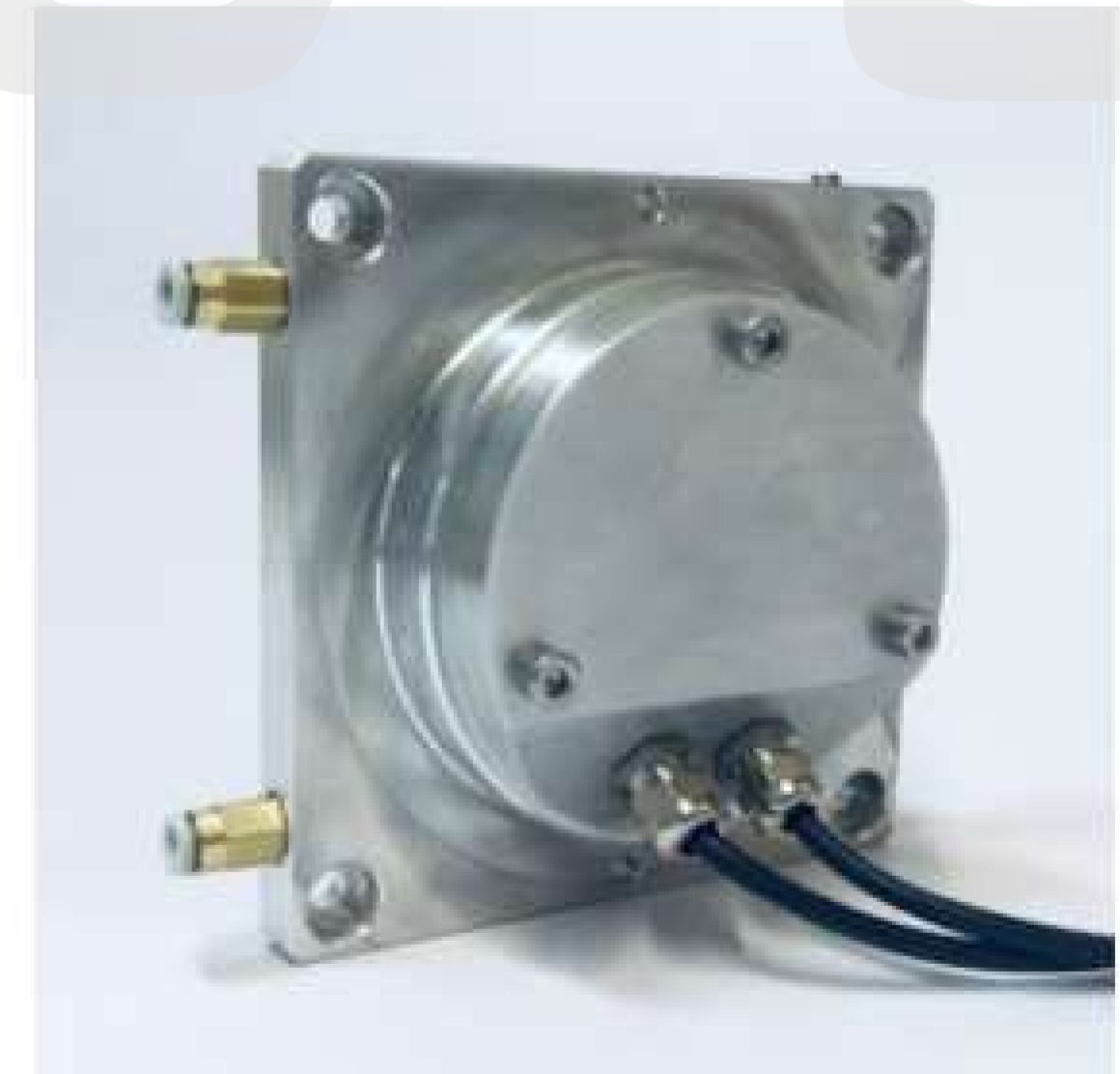
Rear surface of the Zwobbel ® -532 with control and high voltage interfaces.
