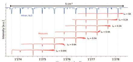
Example of wide scanning of a N20 gas cell, with fast  $I_1$  scans and independent I<sub>T</sub> values.
