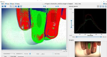
The 4250 system includes proprietary application software featuring fast and easy hyper-cube capture and intuitive image classification/segmentation as part of a suite of powerful spectral image exploration tools.
